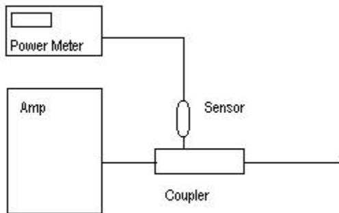
The sensor connects to the forward (or Incident) port of the directional coupler. The power from the amplifier passes through the coupler, and the forward port of the coupler provides a way to sample the power being delivered by the amp.
